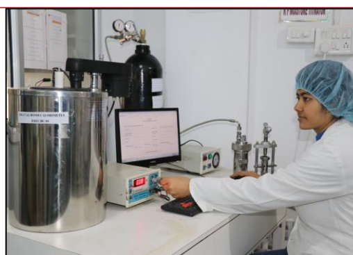
Bomb Calorimeter - Calorific value measurement
